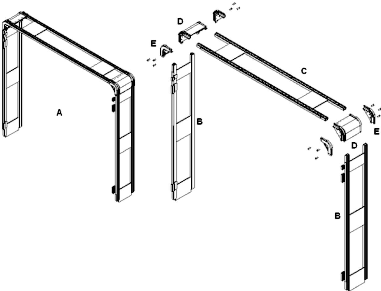
**Table 7.1: Front Bow Assemblies & Parts (Extruded Pull Bar 2006+)**
