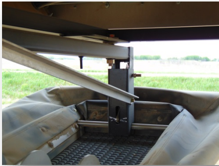
Driver's side lever disengages the passenger side lock to allow the conveyor hopper to lower to ground
