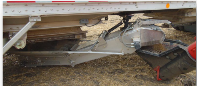
Heavy duty bearings and track allows the conveyor to reach both hoppers
