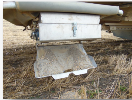
Cleanout is readily accessible.
