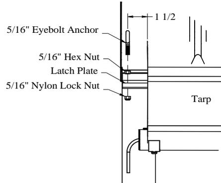
**Step 5:** Insert the Load-Loc Return Rope into the eyebolt, make sure to remove all the slack from rope and knot the rope to prevent it from coming out. Cut off any extra rope and melt the frayed end.
