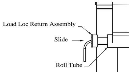
**Step 3:** Gently tap the Load-Loc Return into the roll tube if necessary. Drill a 9/64" hole through the roll tube 7/16" from the edge of the rope guide. Fasten together with a #8 self-tapping screw.
