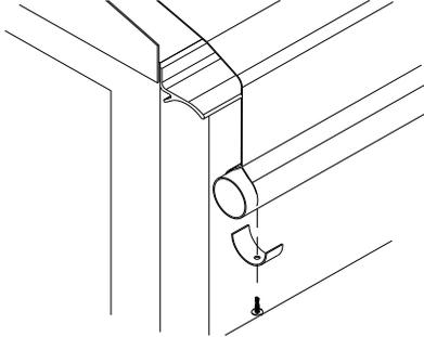
**Step 2:** Insert the Load-Loc Return assembly into the main roll tube.
