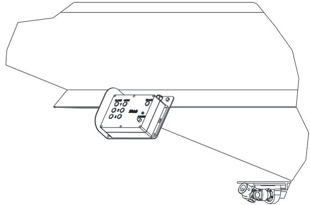
Mount the control box to the shielding mount bracket using the #10 x 1" machine screws supplied.
